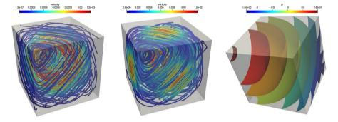
Fig. 1 Example 2: Approximate solutions computed using the MINI-element. Velocity streamlines (left) vorticity streamlines (centre) and pressure distribution (right)
