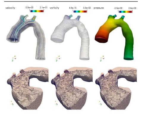
**Fig. 3** Example 4: Simulation of stationary blood flow in an aortic arch. Approximate velocity, vorticity, and pressure (top panels), and samples of adaptive mesh after one, two and three refinement steps, and visualising a cut focusing on the boundaries (bottom row)
